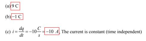
18. A new type of device appears to accumulate charge according to the expression  $q(t)=10t^2-22t$  mC (t in s).
